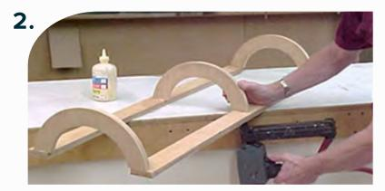
Attach horizontal ribs using glue and staples.
