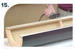
Use a router to remove excess material. Sand/file rough edges.
