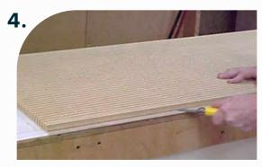
Use a blade to remove one or two ribs. This will allow for a clean insert attachment to framework.
