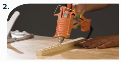
Cut a  $\frac{3}{4}$ " wide seam rib using solid wood or particle board. Apply adhesive to seam rib.
