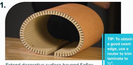
edge to maintain consistent rib spacing. Put decorative surface together and clamp in place.
