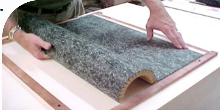
Apply contact adhesive to the face material of the Soflex panel. Place in jig.
