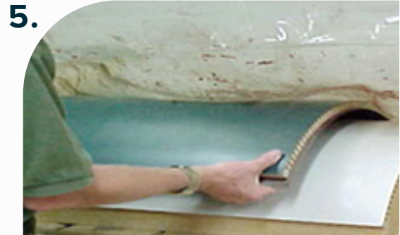
5. Place veneer face down on form. Then, place Soflex with glued rib side down onto veneer.
