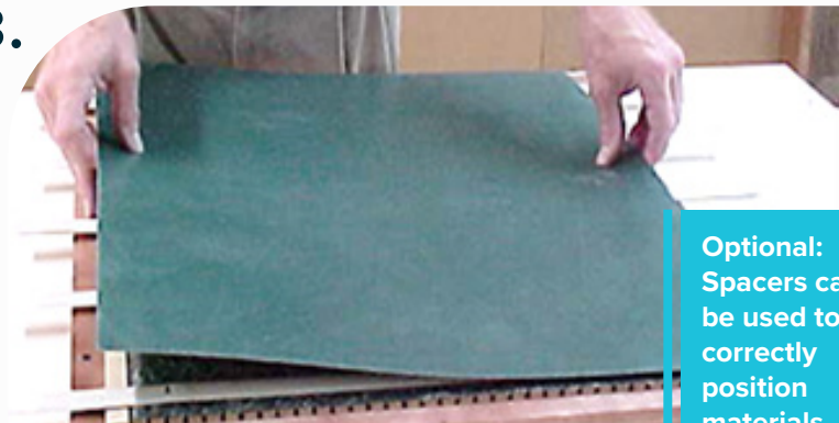
Apply laminate to Soflex
