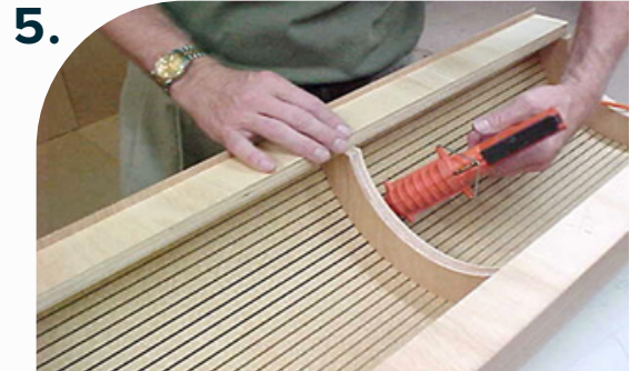
Use hot melt along ribs to help hold in place until the PVA glue sets.
