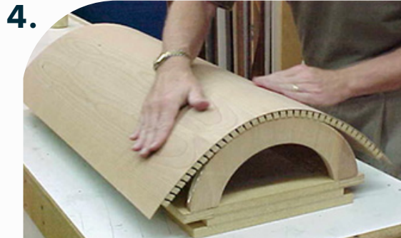
Apply moderate pressure across the entire surface to ensure Soflex attaches to frame.
