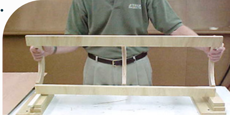
Outfit frame using horizontal ribs.
