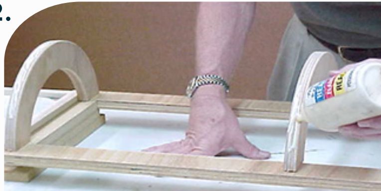
Apply PVA/White glue adhesive outside face of horizontal ribs.
