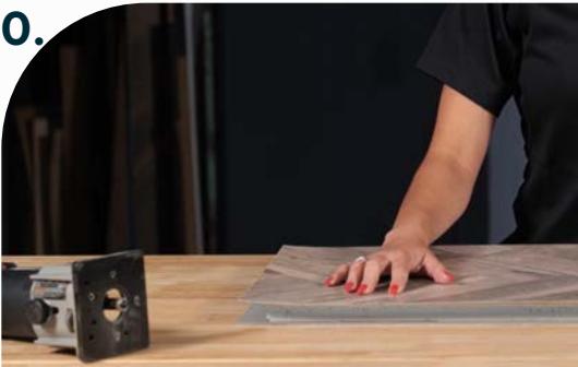
Trim edges using a router.
