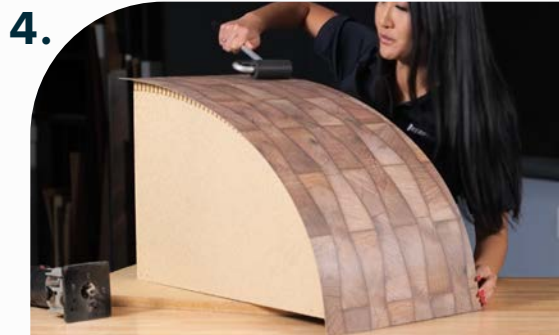
Use a J-Roller to ensure uniform adhesion.
