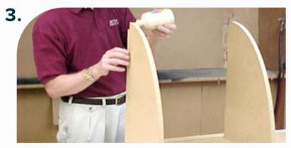
To attach Timberflex the framework should consist of horizontal ribs.
