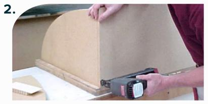
Glue, screws and staples are all suitable for construction.
