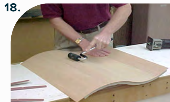
Use a J-Roller to ensure adhesion.
