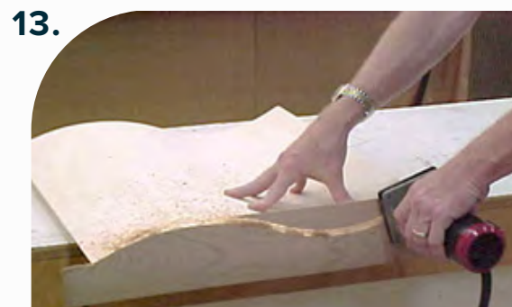
Apply edgework. Trim excess material.
