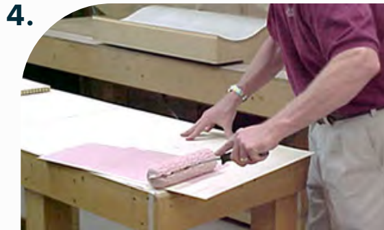
Apply PVA/Wood glue evenly to the back panel.
