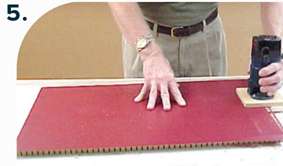
Trim edges using a router.
