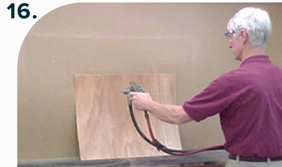
Apply contact adhesive to decorative material.
