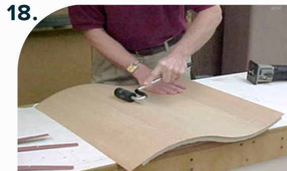
Use a J-Roller to ensure adhesion.
