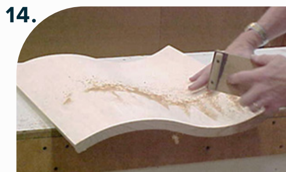
Use sandpaper to smooth rough edges for a clean finish.
