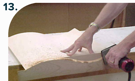
Apply edgebanding. Trim excess material.
