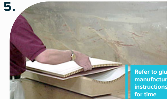
Position Flexboard and back panel together over form.
