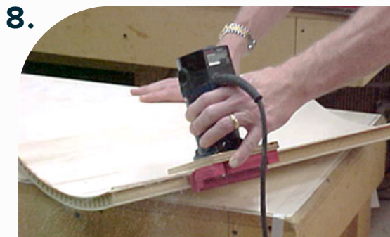
Trim excess material from edges.
