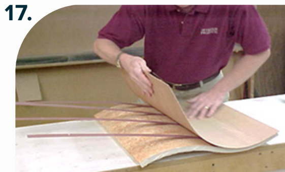
Position decorative material on door.
