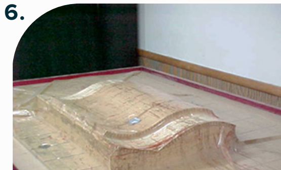
Use vacuum press until dry cycle is complete.
