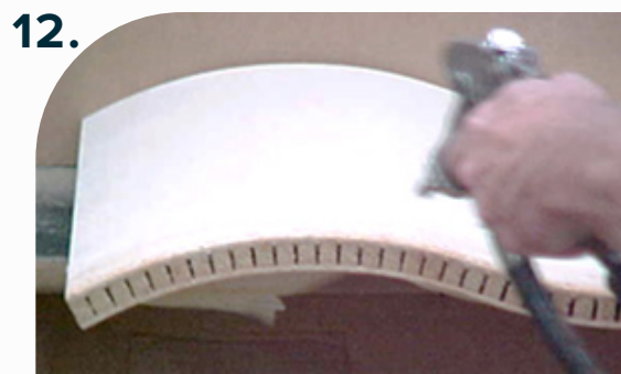
Apply adhesive to panel edge. Mask entire face to prevent glue overspray.
