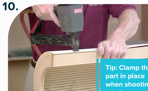
10. Reinforce by shooting staples through the material face into framework.
