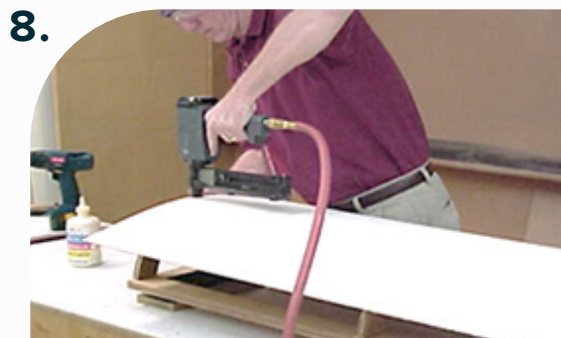
Attach by shooting a narrow crown staple through the face of the material into the support ribs.
