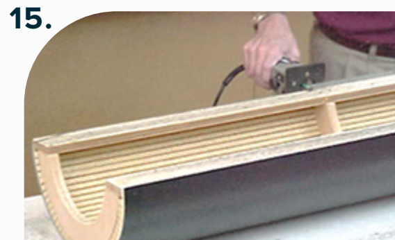
15. Use a router to remove excess material. Sand/file rough edges.
