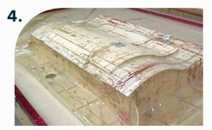
Use vacuum press, straps, or reverse forms to hold shape until dry.
