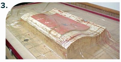
Hold down using a vacuum press or straps until dry.
