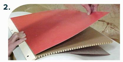
Apply adhesive to each side of the Econokore panel and the back sides of each laminate. Align your laminates and Econokore over the form.
