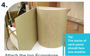
Attach the top Econokore panel to the formed panel. Clamp into position until dry.
