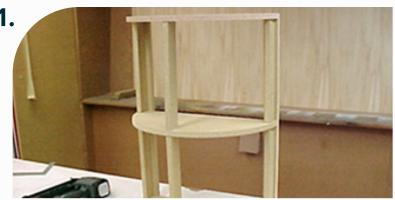
Construct a predetermined framework to create the desired radius.
