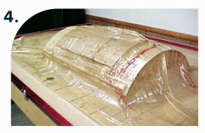
Use a Vacuum Press or Straps to hold the shape until the glue has dried.
