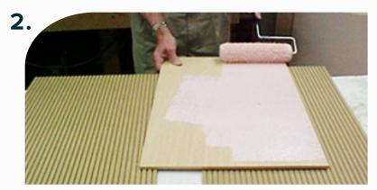
Apply PVA/Wood glue to both sides of the bendable panel or the back side of each Econokore panel.
