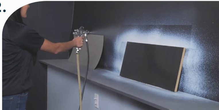
Apply adhesive to both the decorative surface and Soflex substrate.
