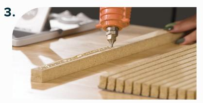
Cut a <sup>3</sup>/<sub>4</sub>" wide seam rib from solid wood or particleboard. Apply adhesive to seam rib.
