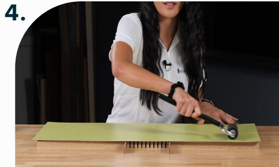
Apply pressure with a J-Roller to ensure good adhesion.
